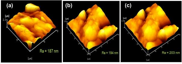
Figure 2. AFM Topography of NK membranes (a) NK34, (b) NK35.5 and (c) NK37.
