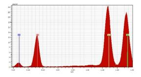
**Figure 1.** EDX spectra of the fabricated membrane showing: Oxygen (O), Aluminum (Al), Silica (Si) and Carbon (C)
