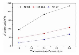
**Figure 3.** Effect of Transmembrane Pressure on oilwater flux of NK based different concentration membranes.
