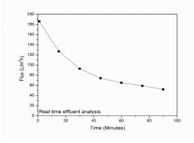
**Figure 6.** NK37 membrane flux performance of real time oil-water effluent (Transmembrane Pressure-3 bar).
