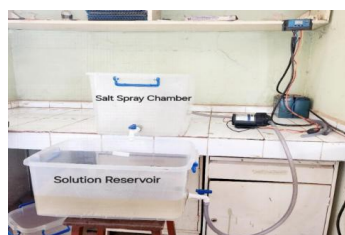
Figure 1: Fabricated laboratory salt-spray accelerated corrosion testing setup showing the salt spray chamber (upper container) and solution reservoir (lower container) connected through a pumping system used to generate a continuous saline mist for coating durability evaluation under simulated marine conditions.
