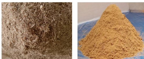
Figure 1: Saw dust samples preparation- Free saw dust and powdered Sawdust respectively
