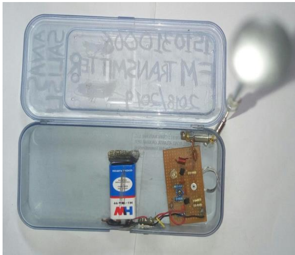
Figure 4. The constructed FM transmitter during test
