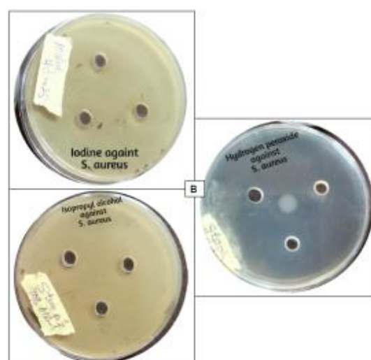
Plate B: Petri dishes showing the zone of inhibition against S. aureus .
