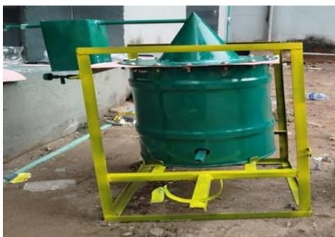
Figure 4: HDPE torrefaction reactor
