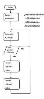
Figure 1. Voltmeter, Ammeter and power Flow Chart.
