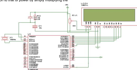
Figure 4. The Designed Circuit Showing PIC and LCD Connections
