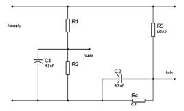
Figure 2. Voltage Divider Attenuator Circuit
