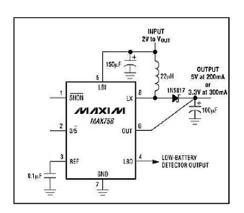
Figure 2. Circuit diagram using the setup chip [7].
