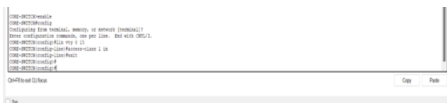
Figure 26: ACL activated on the core switch to authorize only the engineering hosts.
