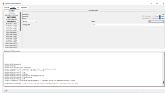
Figure 10: Ports connected to the Rogue PC-1 disabled.
