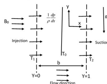
Figure 1: Geometry of the Flow System
