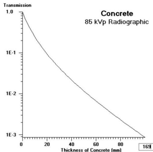
**Figure 4:** Attenuation curve for console of Specialist hospital Sokoto (Generated from the XRAYBARR).
