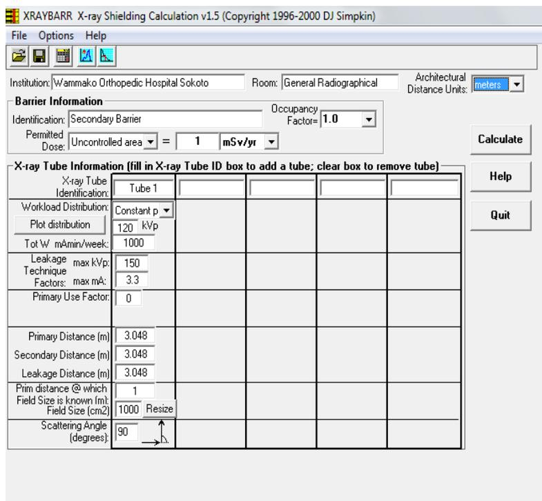
Figure 2: XRAYBARR Software Interface [11].
