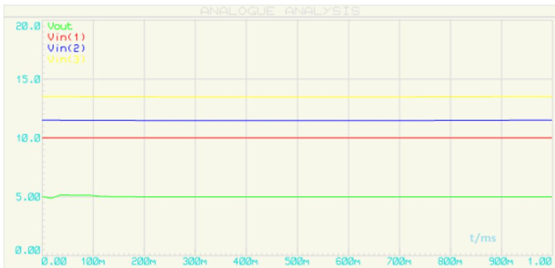
**Figure: 8** Simulations of the Voltage Regulator Stage in Proteus
