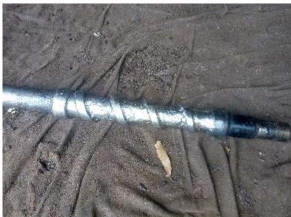
**Figure 2:** Locally Fabricated Worm Screw
