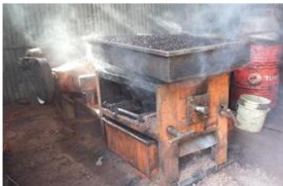
**Figure 1:** Locally Fabricated Palm Kernel Screw Press.
