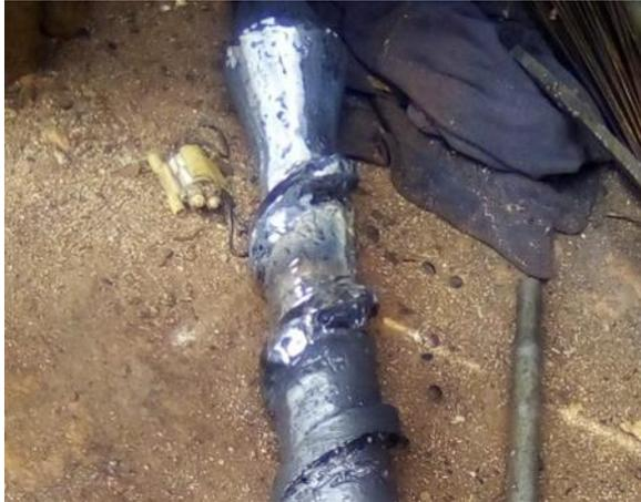
**Figure 4:** Failed Worm Screw
